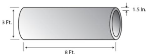
Steel tube weight = 9.03 cubic feet x 480 pounds per cubic foot
