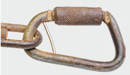
Missing / modified / improperly replaced fasteners
