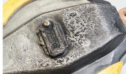
Heat damage (burns / weld splatter)
