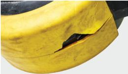
Damage to casing / nicks / gouges
