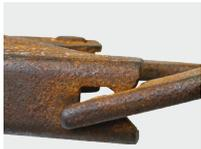
Distortion (bent / twisted / stretched)
