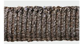
Heat damage (burns / weld splatter)
