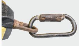
Distorted hardware (bent / twisted / stretched)
