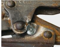
Heat damage (burns / weld splatter)
