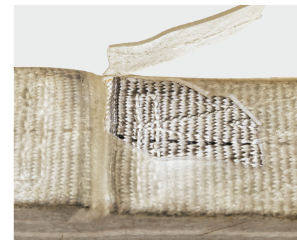
Open / torn cover
