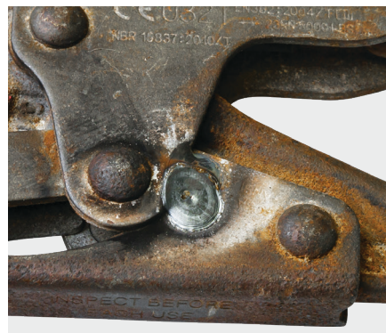
Heat damage (burns / weld splatter)
