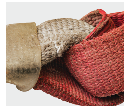
Torn / frayed webbing
