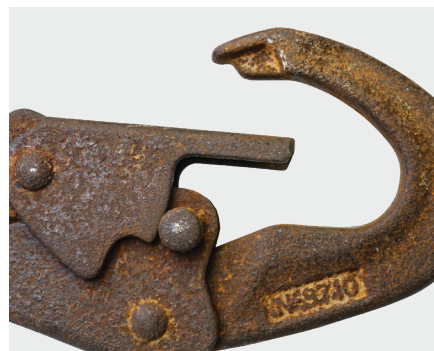
Hardware / gates that do not freely move
