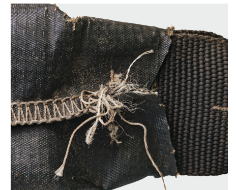
Ripped / missing stitching
