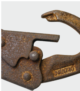
Hardware / gates that do not freely move
