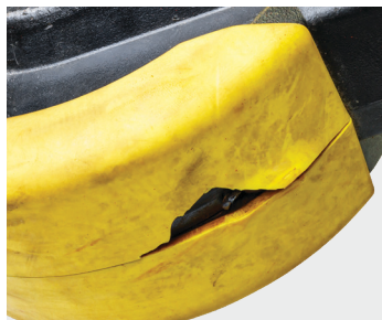
Damage to casing / nicks / gouges
