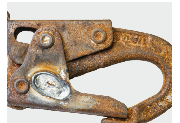
Hardware / gates that do not freely move
