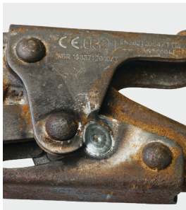
Heat damage (burns / weld splatter)
