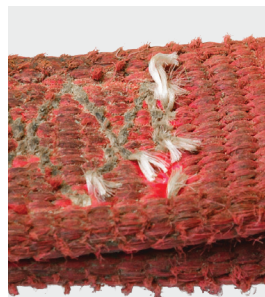
Loose / frayed stitching
