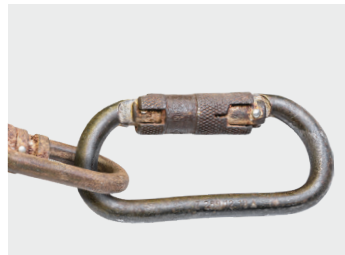
Distorted hardware (bent / twisted / stretched)
