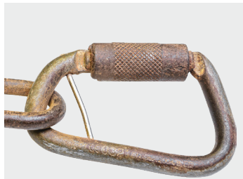
Missing / modified / improperly replaced fasteners
