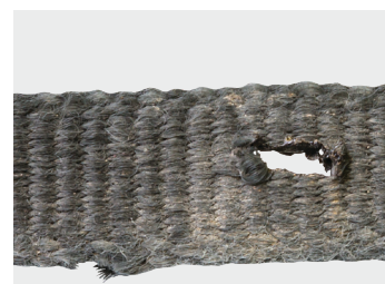
Cuts / holes / punctures
