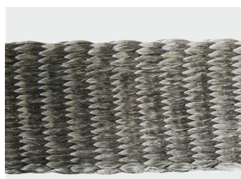
UV damage / discoloration
