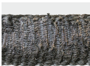
Abrasion / wear / deterioration
