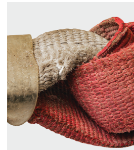
Torn / frayed webbing
