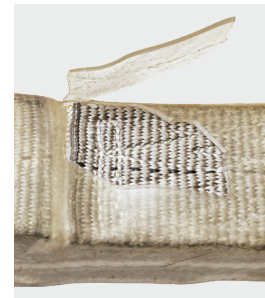
Open / torn cover
