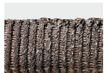
Heat damage (burns / weld splatter)
