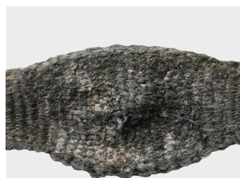
Distortions / crushed webbing
