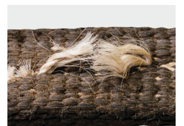
Loose / frayed stitching
