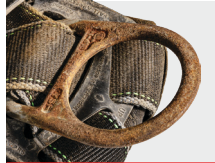
Corrosion of D-ring or fasteners
