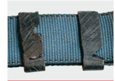
Loose / damaged mountings
