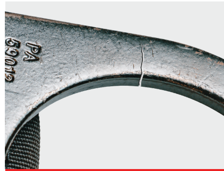
Cracks in D-ring or fasteners
