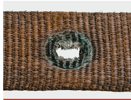
Grommets not secure (wiggling) or missing
