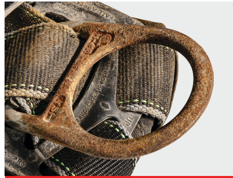
Corrosion of D-ring or fasteners
