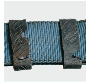
Loose / damaged mountings
