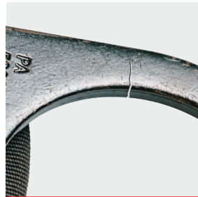
Cracks in D-ring or fasteners
