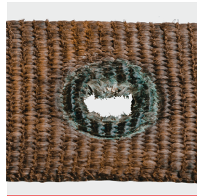
Grommets not secure (wiggling) or missing
