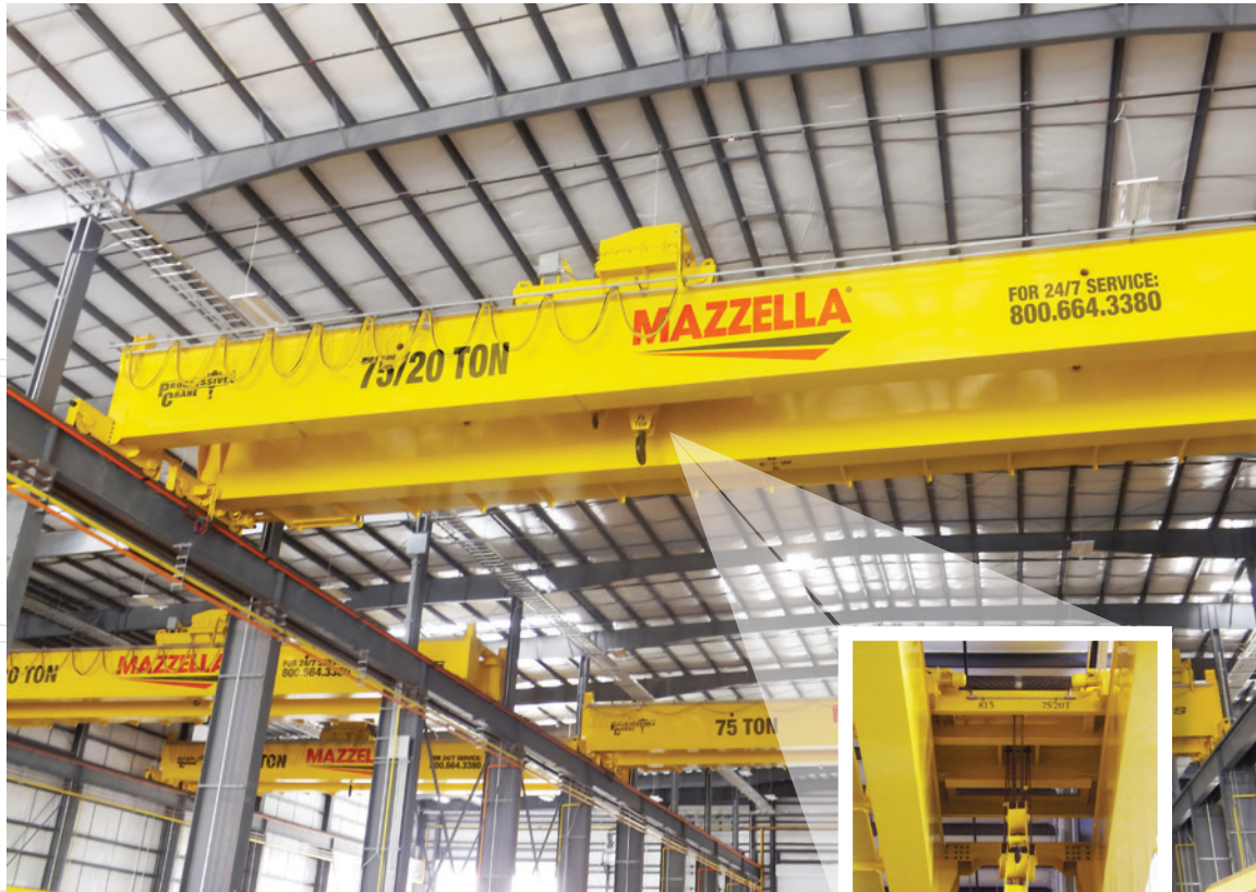
Top running, double girder cranes with auxiliary hook.
