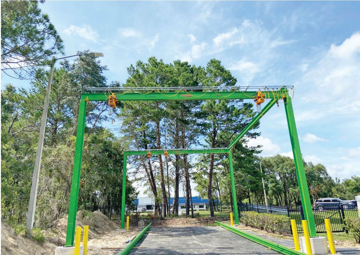
Crane used for covering loads on flatbeds.
