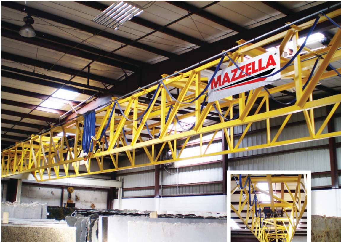
Trussed-style bridge for extremely long span.
