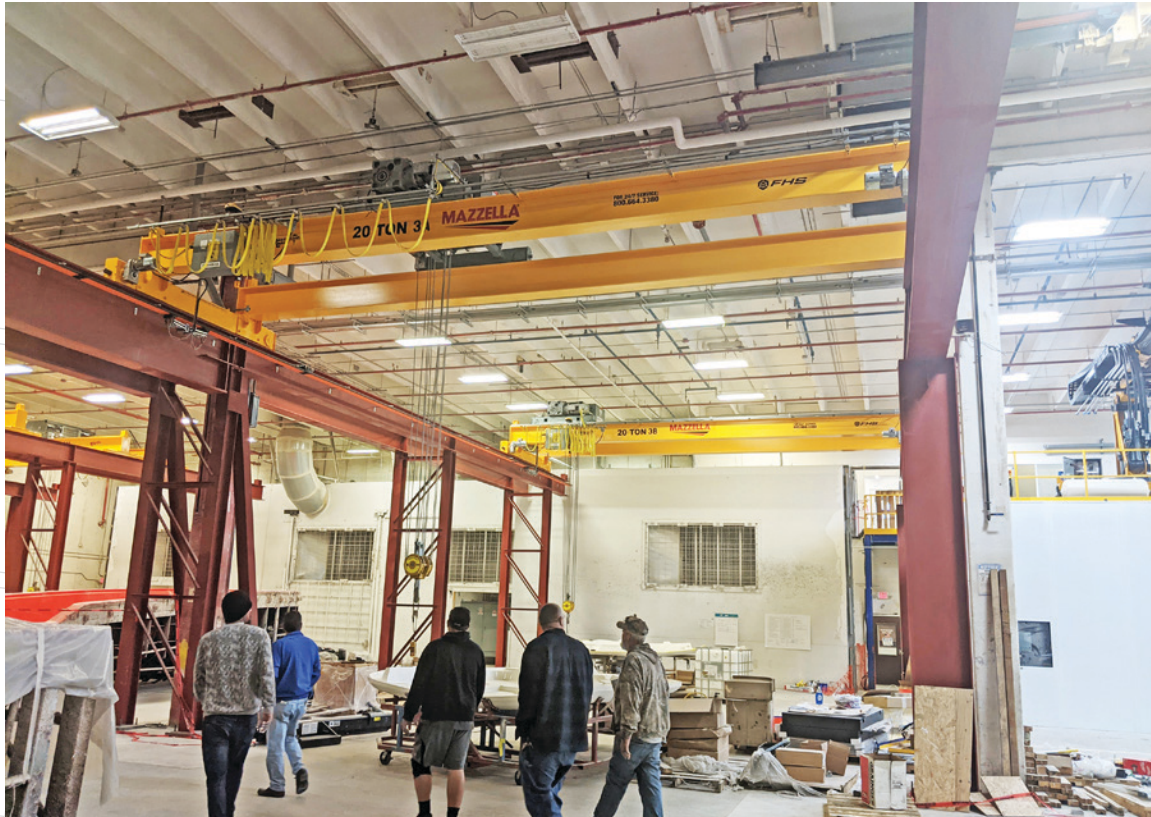
Multiple crane system with latted columns and longitudinal A-Frames
