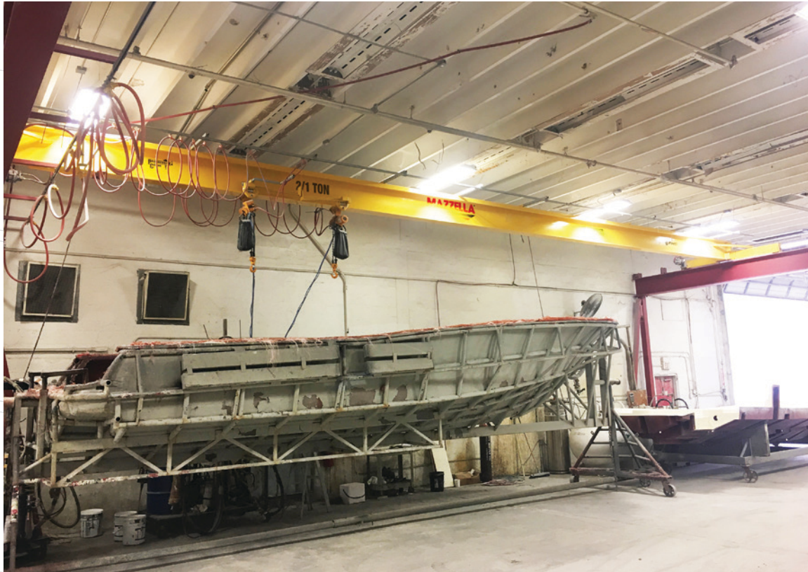
Pneumatic crane for flammable environment.
