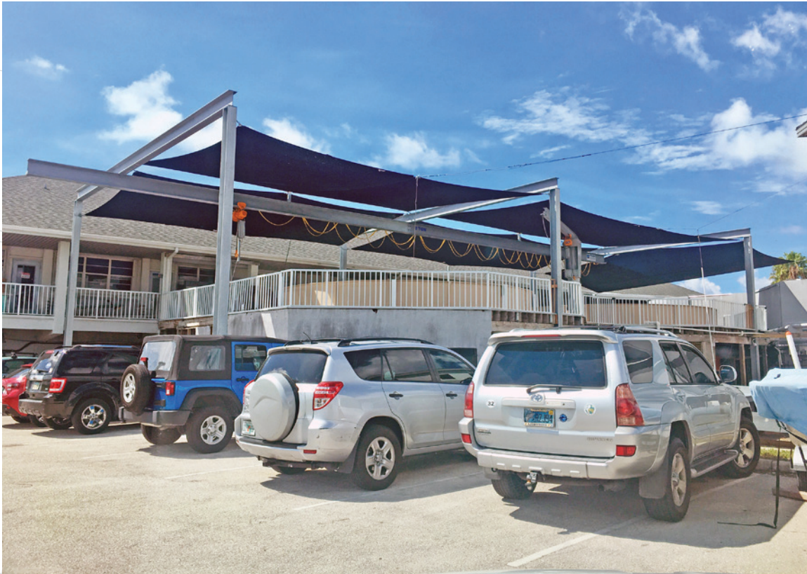
Galvanized monorail crane with sun shade for outdoor marine environment.
