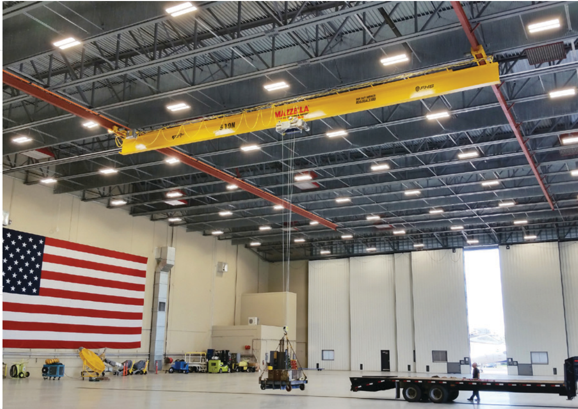
Underhung crane used for aircraft maintenance.
