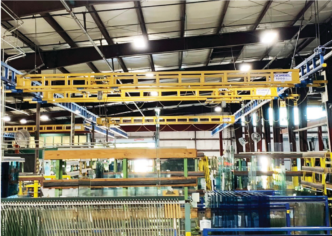
Workstation cranes with “nested trolley”.
