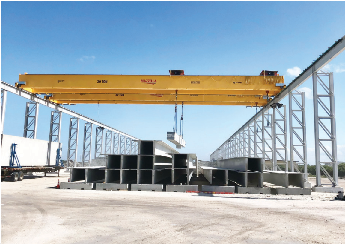
Outdoor crane system for storage and loading onto flatbeds.
