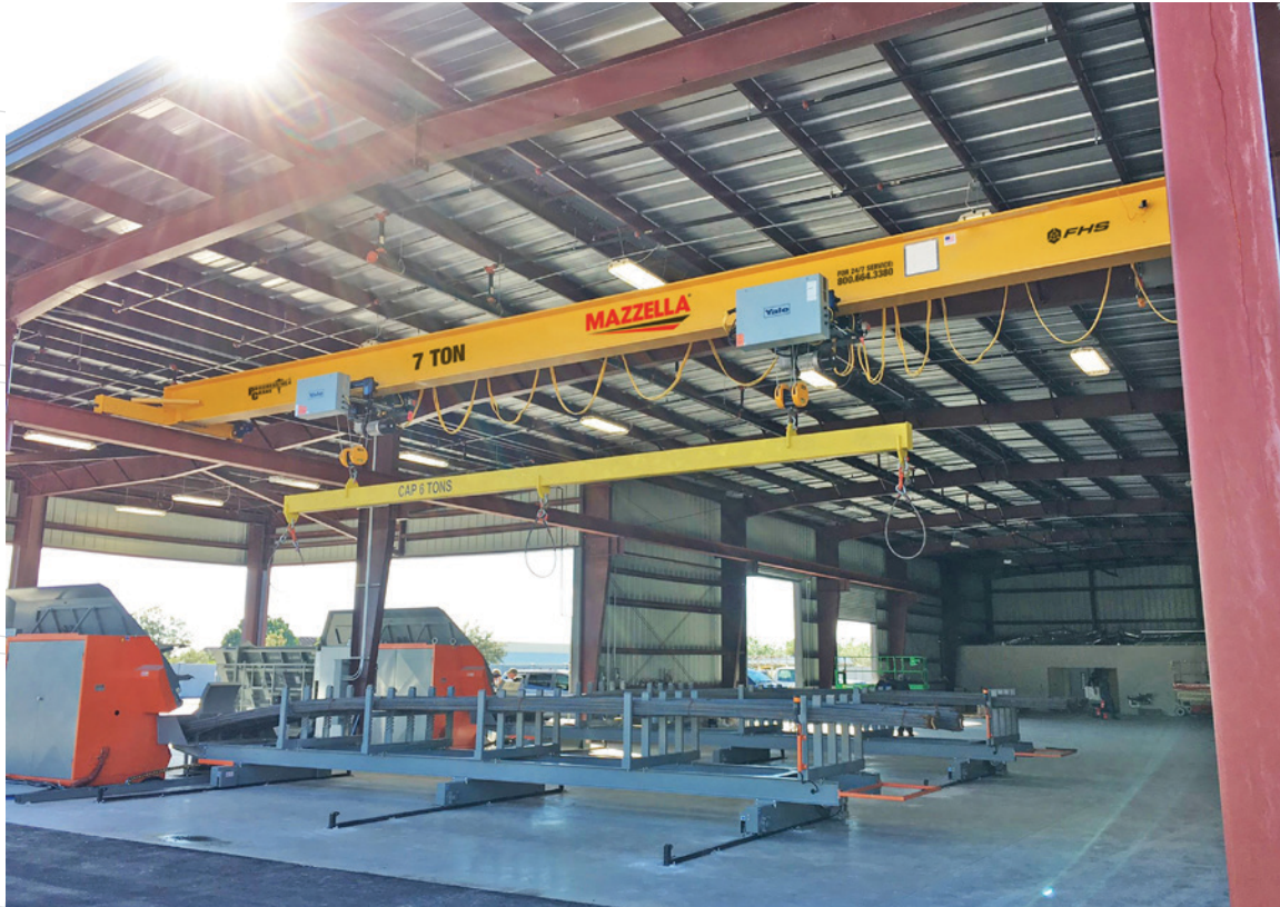
Dual hoist crane system with a 3-point spreader bar for long loads.
