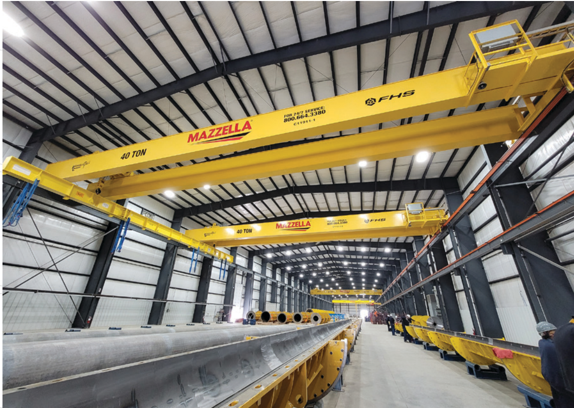
Double girder cranes lift in tandem, wall-sliding jib crane as auxiliary.
