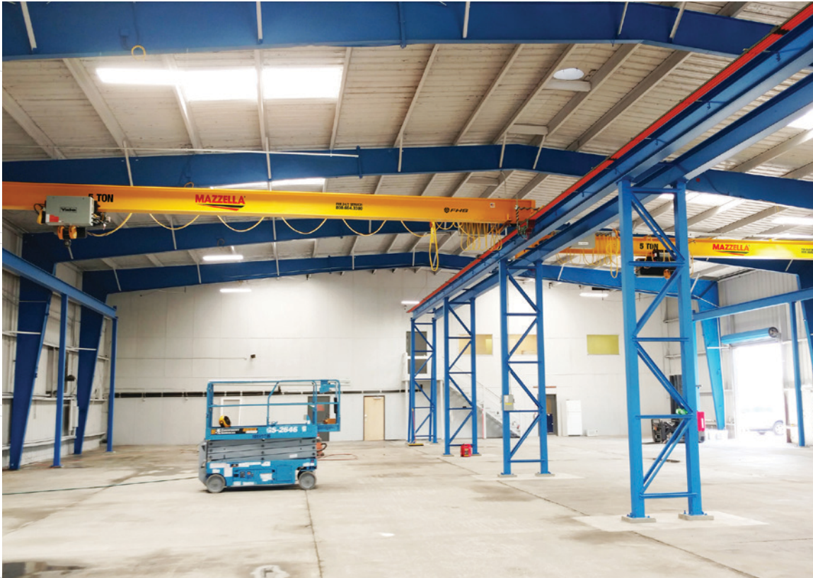
Side-by-side cranes with common center columns.
