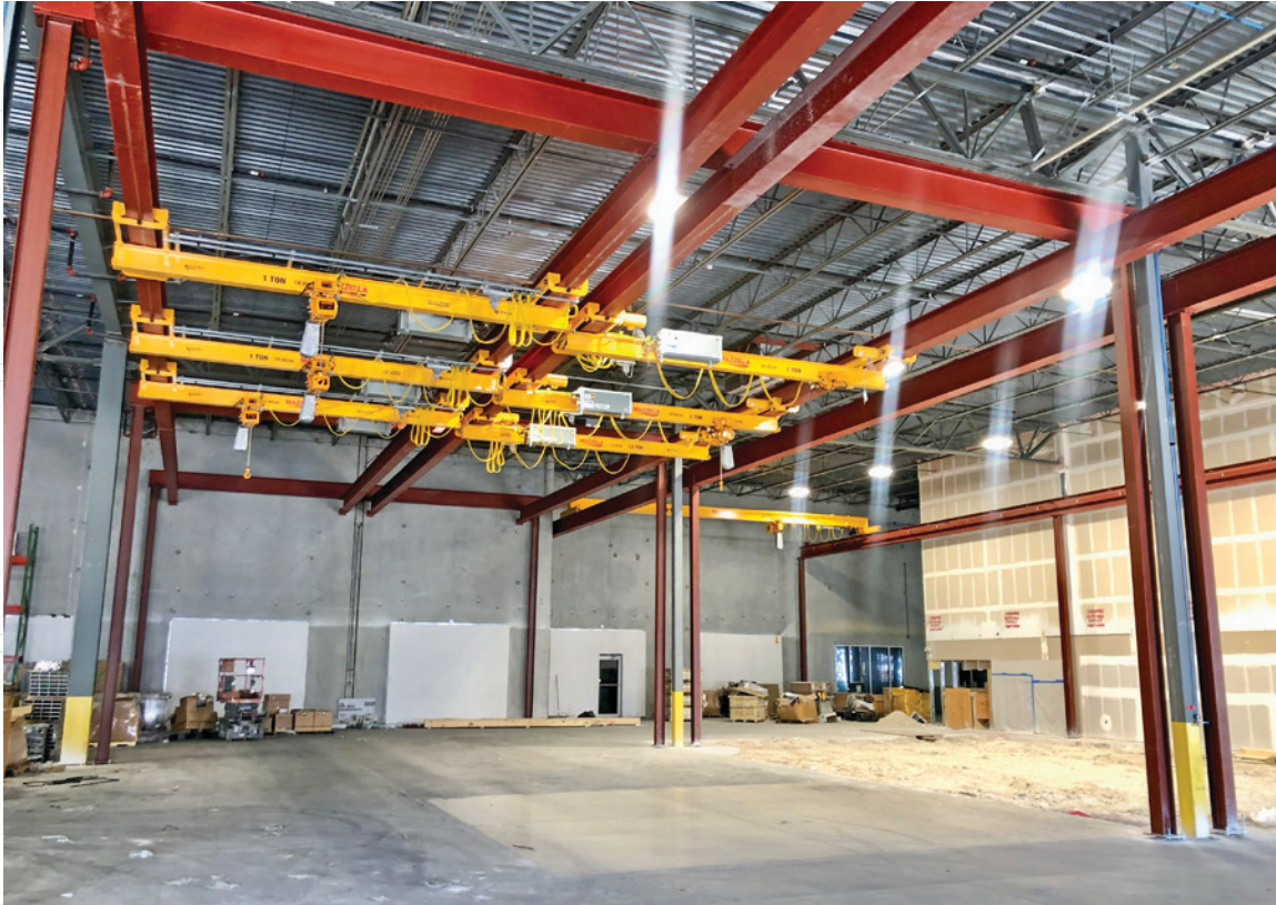
Underhung cranes for side-by-side production lines.
